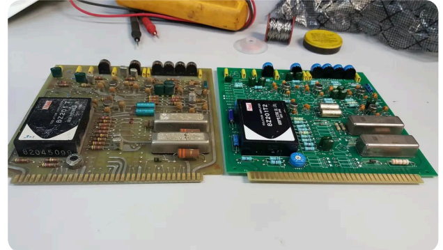
Drive boards on the bench for component-level repair.
